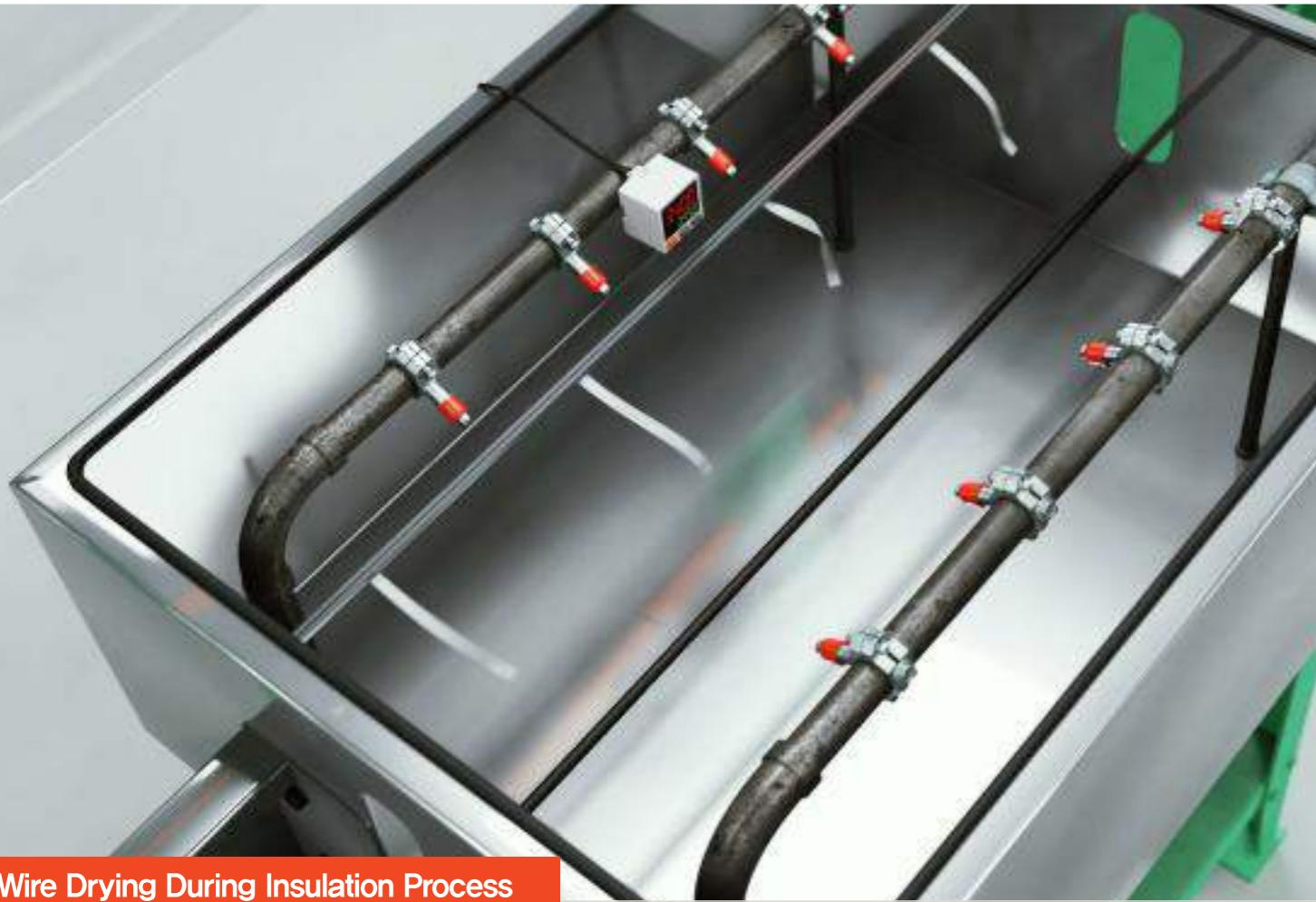
Wire Drying During Insulation Process
