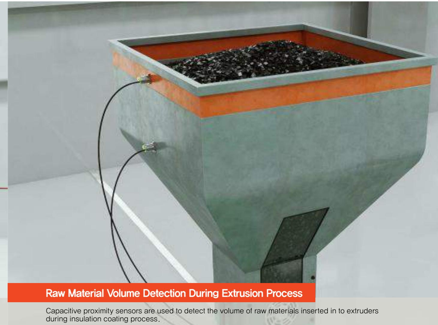
**Raw Material Volume Detection During Extrusion Process**
