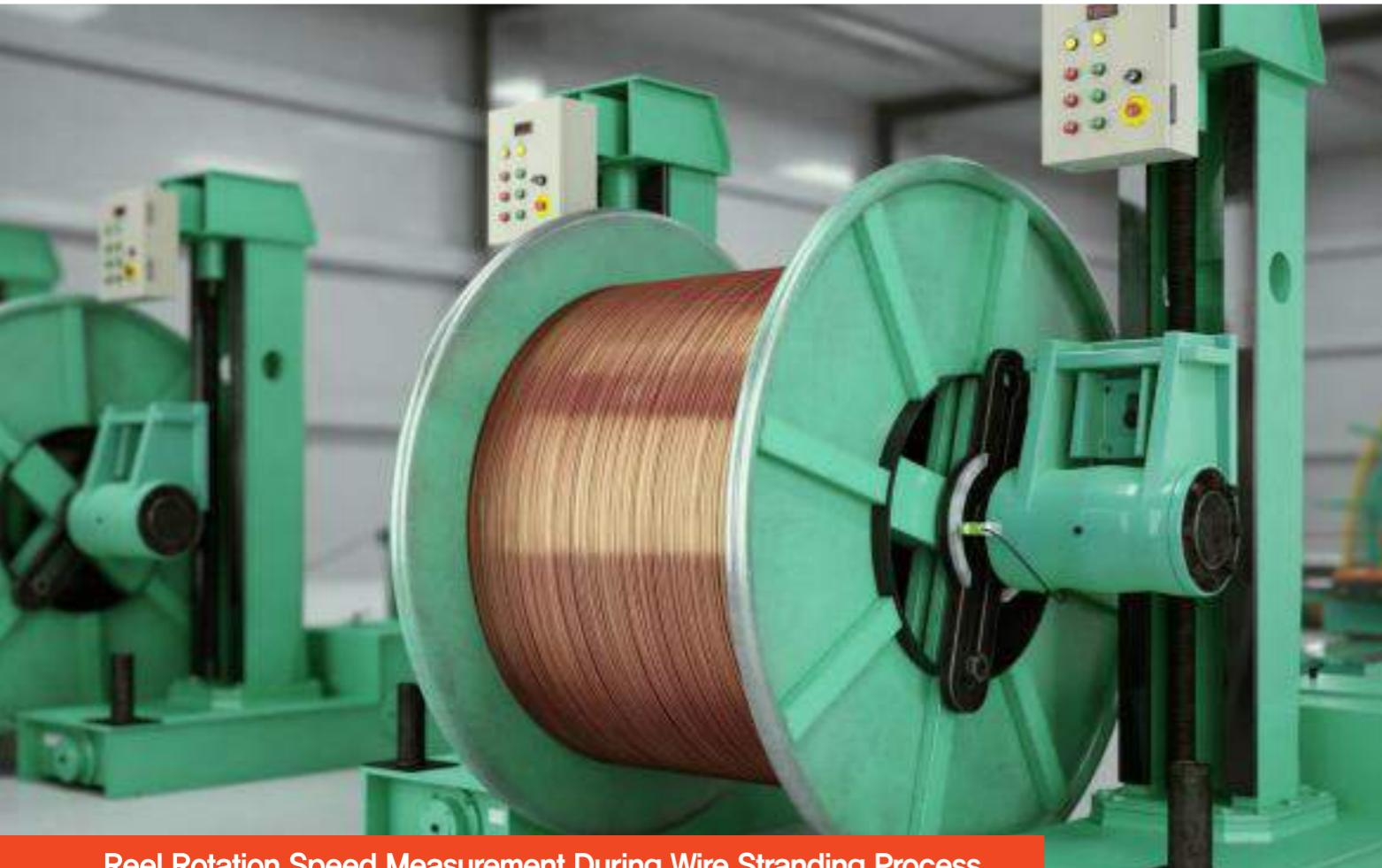
**Reel Rotation Speed Measurement During Wire Stranding Process**
